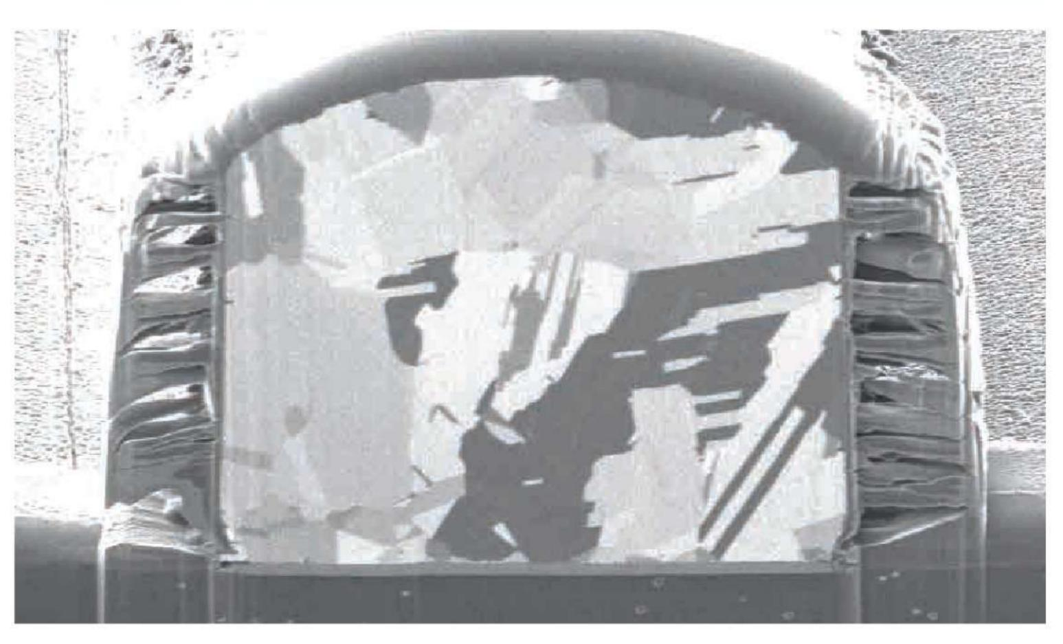
Electrolytic Cu plating: 8 µm (1.5 ASD)
