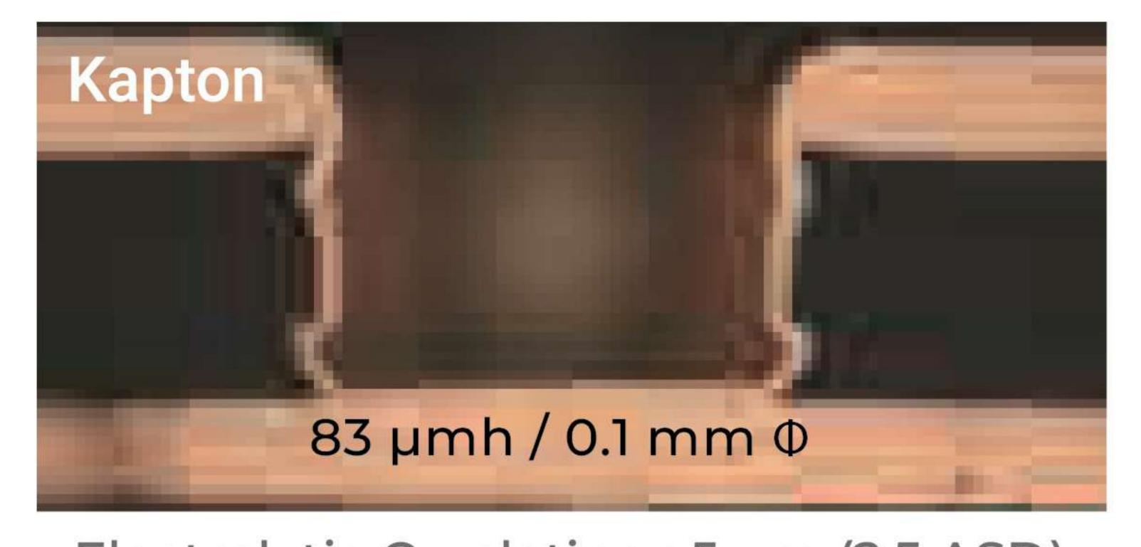
Electrolytic Cu plating: 5 µm (2.5 ASD)
